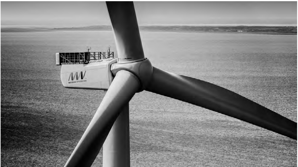
Figure 20: Vestas V164-8MW - the largest (offshore) wind power turbine available
